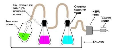
Alternatively, a commercially available vacuum trap, such as the Guardian canister can be used.
