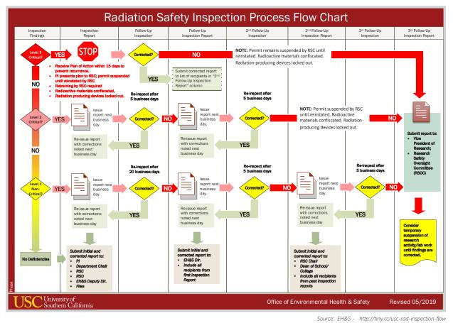
Figure 5.1. Radiation Safety Inspection Process Flow Chart
