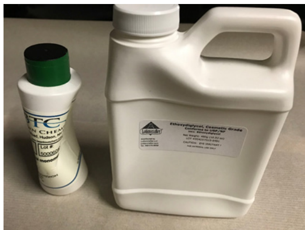
Figure 7.9. Polyethylene containers on prolonged storage of organic peroxide formers
