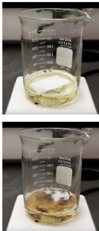
Figure 9.3. Piranha solution with paper strip. Top: Start. Bottom: After a few moments.
